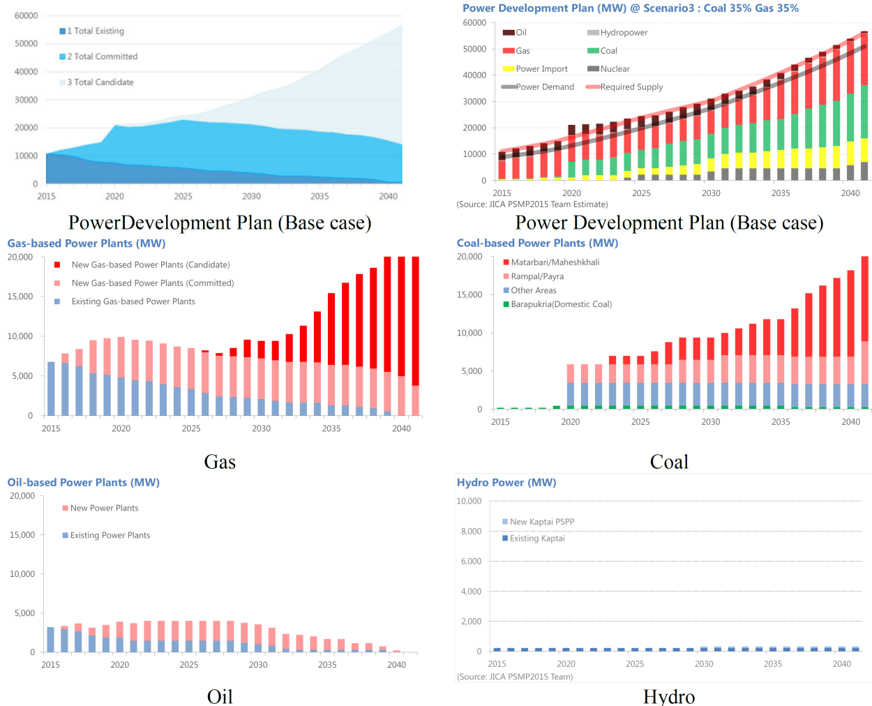
Figure 11: Bangladesh – Development of power generation capacities under SCENARIO 3 of the PSMP 2016
